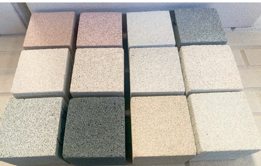
AAC sample blocks produced from different solid wastes as raw materials.
